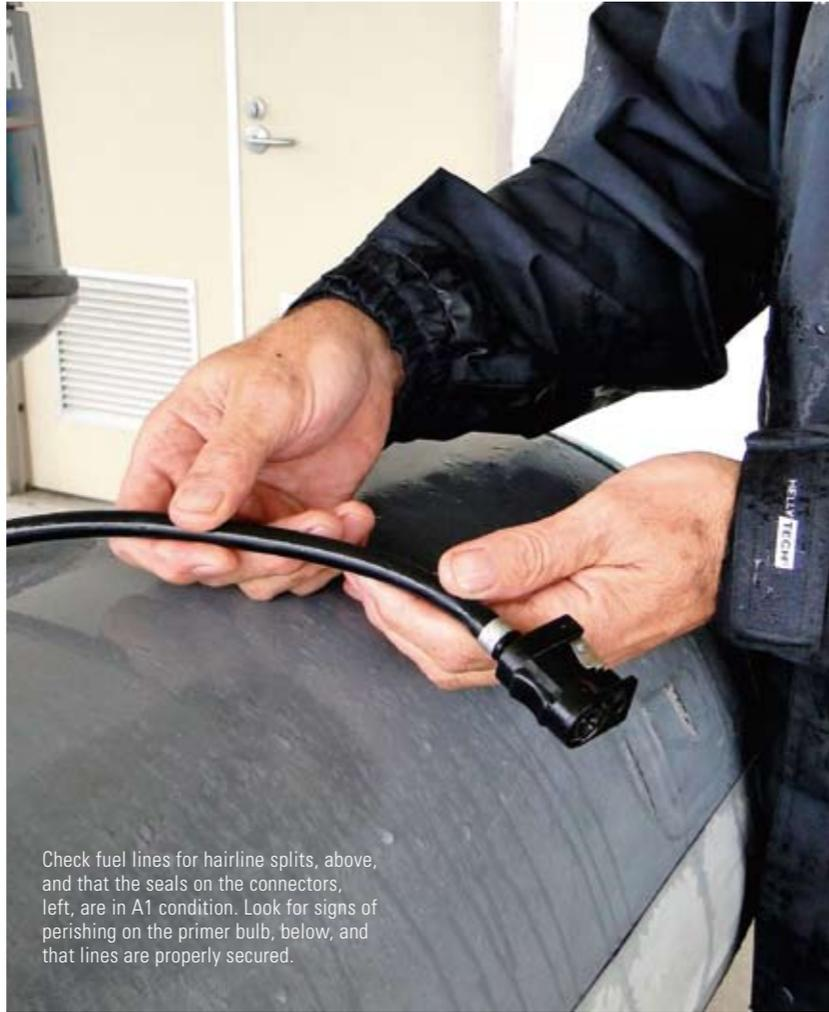
Check fuel lines for hairline splits, above, and that the seals on the connectors, left, are in A1 condition. Look for signs of perishing on the primer bulb, below, and that lines are properly secured.
