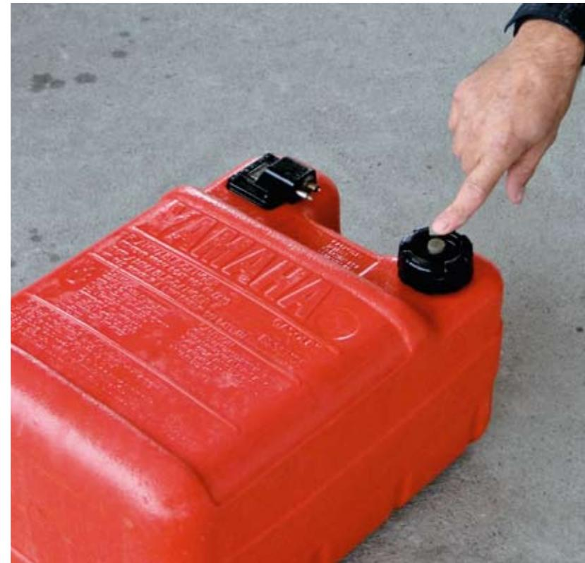
Above: It is mandatory by law to remove tote tanks from boats for refuelling. Left: Filler caps have an air-release screw that must be closed when the fuel tank is not in use.
