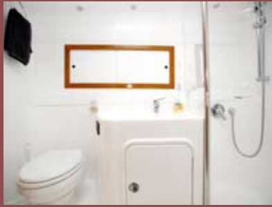
Above: Moulded fibreglass head features an electric loo, shower and vanity unit. Right: Flybridge helm station has a low moulded dash with Raymarine E120, and great sight lines to the bow and back to the transom.
