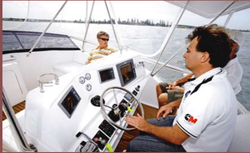
Above: Moulded fibreglass head features an electric loo, shower and vanity unit. Right: Flybridge helm station has a low moulded dash with Raymarine E120, and great sight lines to the bow and back to the transom.
